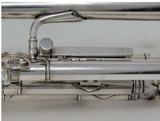
Unique Bb/A stop mechanism
